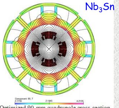
: Optimized 90-mm quadrupole cross-section.
