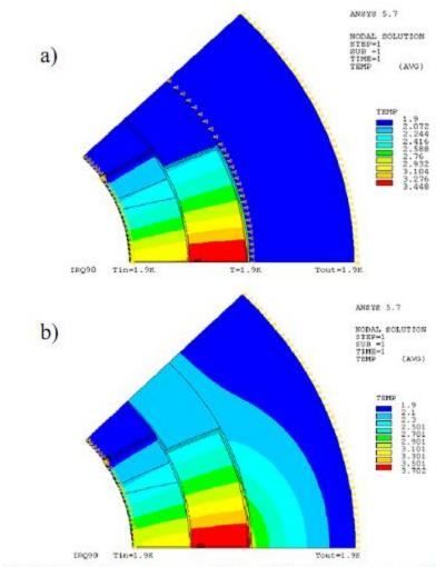
Fig.4. Calculated temperature profile in Nb<sub>3</sub>Sn IR quadrupole without the inter-layer channel for two cases: a) HeII penetrates between collars reaching the coil outer surface; and b) HeII does not penetrate inside collar blocks.
