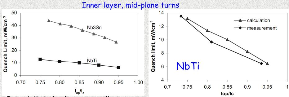
Quench limit (and corresponding magnet operation margin) for Nb<sub>3</sub>Sn is ~4 times larger than for NbTi
