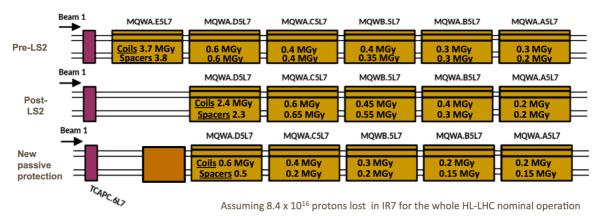
Figure 2 — Summary of doses in different magnets of the Q5 assembly for B1, in the present (top) and proposed post-LS2 (bottom) layouts. The middle plot shows the situation in case no upgrade of the passive collimation system is made. Courtesy of C. Bahamonde [2,3].
