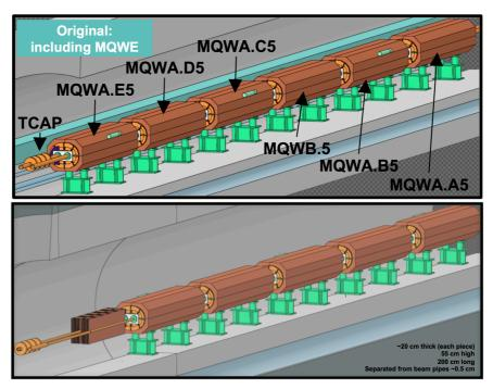
Figure 1 — Illustrative view of the present and post-LS2 layouts of the IR7 Q5 [2,3].
