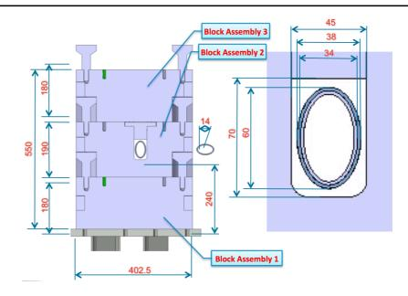
Figure 5 — Cross section of the TCAPM, with the vacuum chambers. Dimensions are given in mm. Courtesy of L. Gentini [8].
