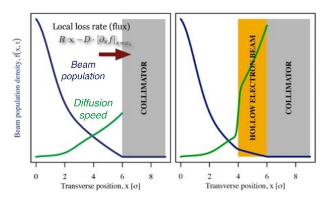
Hollow electron beams provide a possible way to selective (by transverse amplitude) control the particle's diffusion speed and halo populations.
