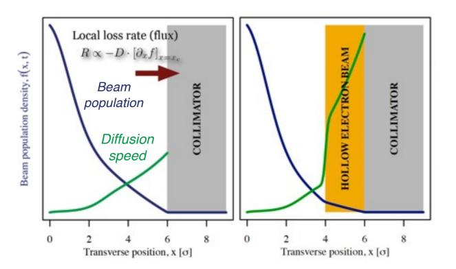
Hollow electron beams provide a possible way to selective (by transverse amplitude) control the particle's diffusion speed and halo populations.
