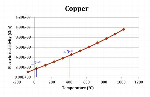
Electric resistivity at 400°C = 2.5 times the one at 27°C
