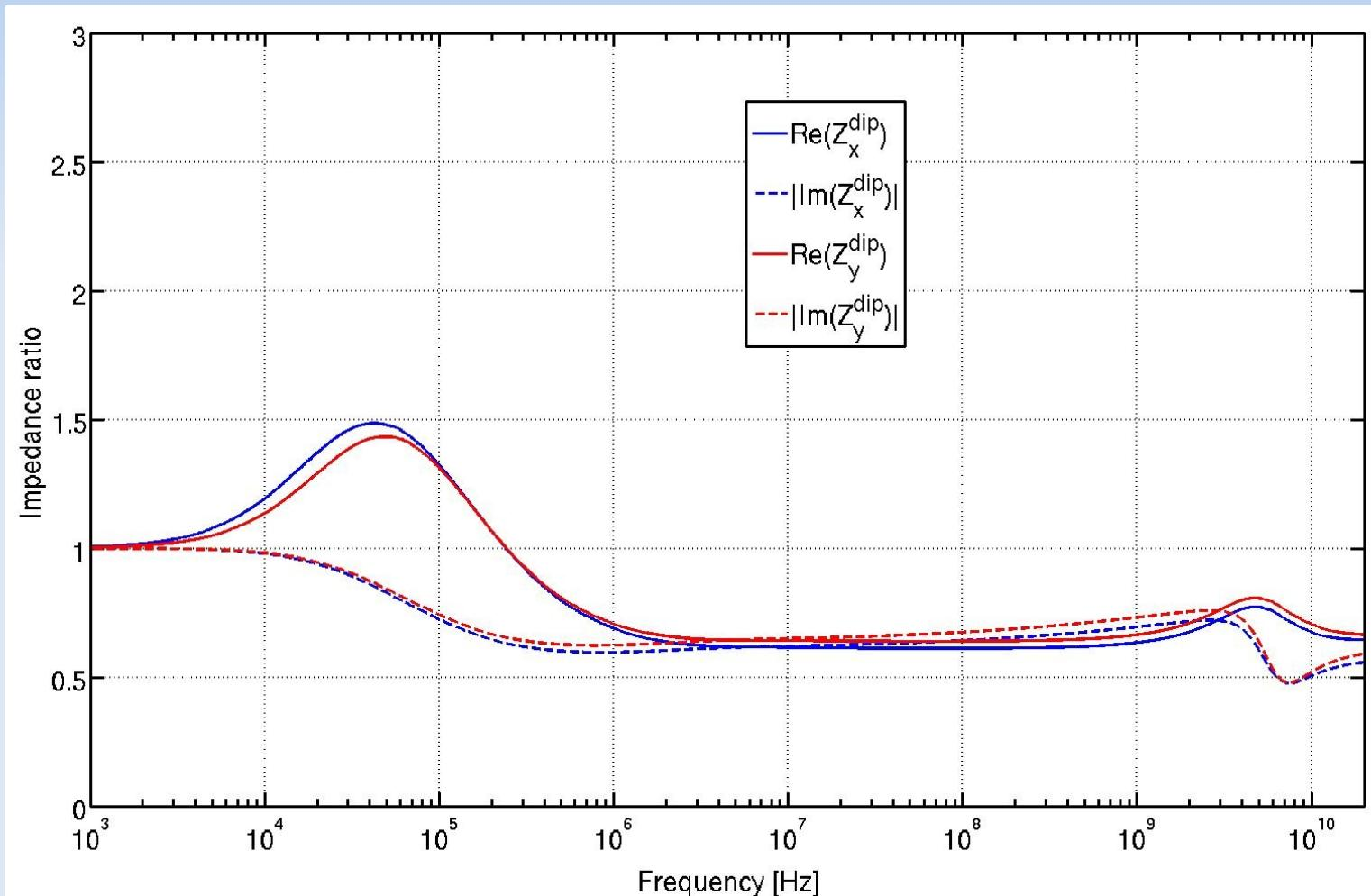
⇒ At intermediate frequencies, we gain **~40 %** with molybdenum.
