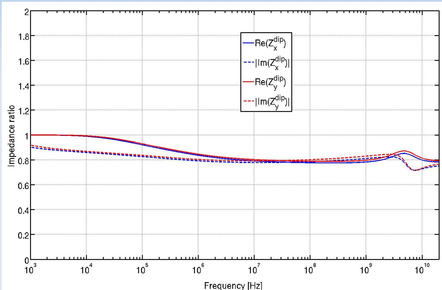
⇒ At intermediate frequencies, gain of only ~20% in impedance.
