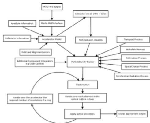
Figure 1: An example logical flow of a Merlin run.
