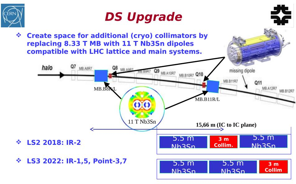
Joint development program between CERN and FNAL underway since Oct-2010 to demonstrate the feasibility of Nb3Sn technology for this upgrade by 2014.
