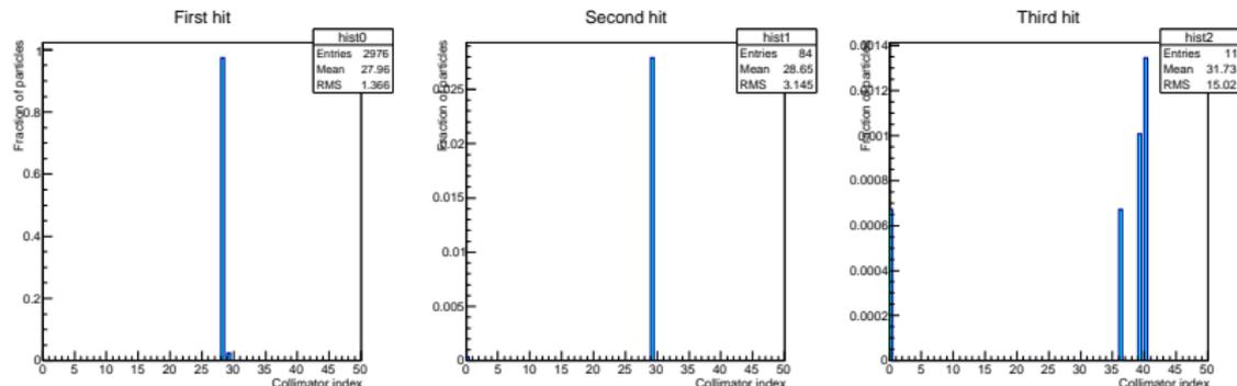
In that case, most of the particles hit just once a primary collimator and just a few hit a second primary collimator. A very few percentage hits also a secondary collimator before hitting the triplet.
