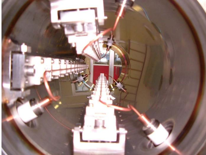
2x2 water-cooled units presently installed in the SPS (two with remote control)
