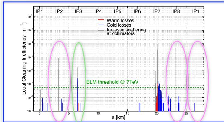
Non linear collimation system in IP7
