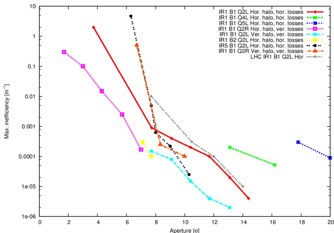
Figure 3: Simulated cleaning losses from SixTrack on different IR magnet apertures, when these apertures were varied. No TCTs are included in the simulation. Nominal collimator settings were used and optics version HL-LHC v1.0. Courtesy of H. Garcia, Royal Holloway University of London.
