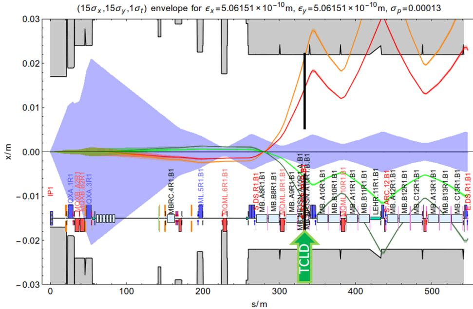
Figure 9: Secondary beams created in Pb ion collisions, shown in the horizontal plane, emerging from IP1 and potentially quenching dispersion suppressor magnets. A collimator installed in the position indicated can intercept the most intense (red) beam. Courtesy of J. Jowett and M. Schaumann.
