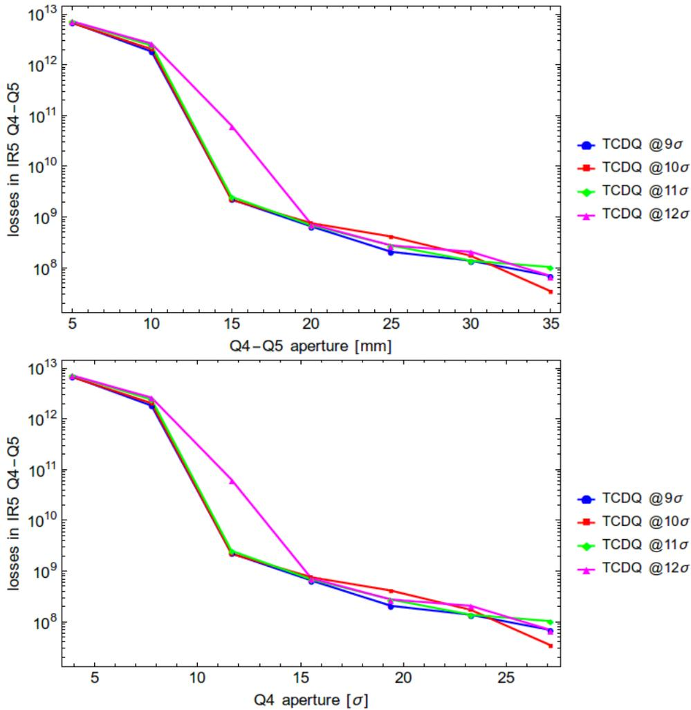
Figure 2: Total simulated losses from SixTrack during an erratic beam dump (single-module pre-fire), normalized to a bunch population of  $2.2 \times 10^{11}$  protons, that are impacting in the Q4 and Q5 in IR5 B2, for different magnet apertures and settings of the TCDQ (dump protection). All other collimators were kept at their design setting, with the primary collimator at  $5.7 \sigma$  and a  $2 \sigma$  retraction in IR7. Optics version HL-LHC v1.0 was used. Courtesy of E. Quaranta, CERN.
