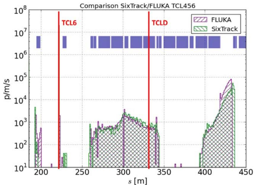
Figure 10: Collisional proton losses around the IR1 DS versus longitudinal position, for FLUKA (purple) and SixTrack (green) simulations, with TCL4, 5 and 6 set at 15, 35 and 10  $\sigma$ . The losses are expressed in protons/m/s, for the design luminosity. The locations of the TCL6 (included) and the possible TCLD (not included in the simulation) are indicated by red lines. Figure adapted from Ref. [24].
