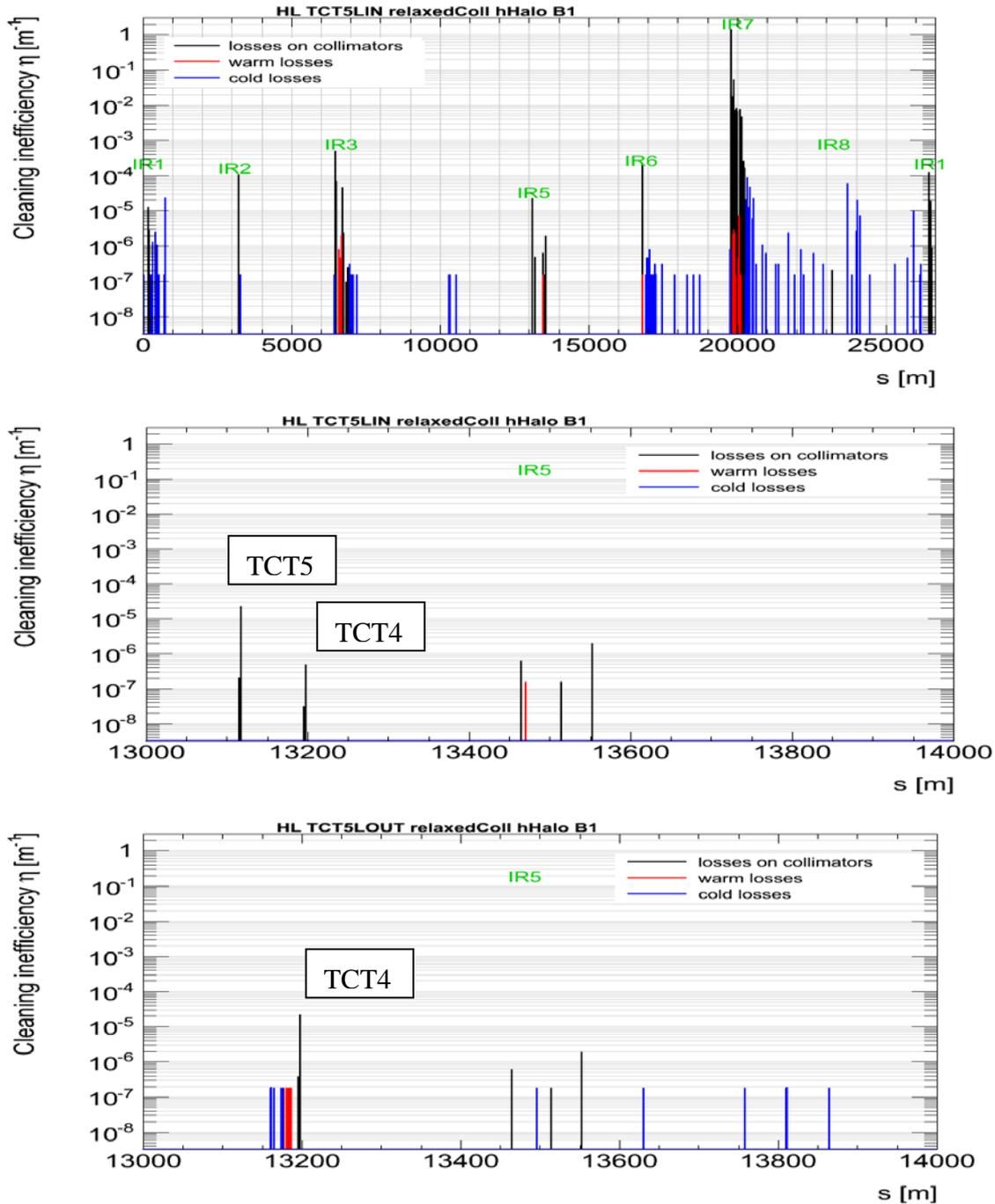
Figure 4: Losses from a horizontal halo in B1, simulated with Sixtrack around the LHC ring (top) and zoomed in IR5 (middle) using the collimation layout for HL with the TCT5 installed. A round  $\beta^*=15$  cm optics (HL-LHCv1.0) was assumed and collimator settings with  $2\sigma$  retraction. The bottom plot shows the losses in IR5 for the same case but without TCT5. Courtesy of R. Kwee-Hinzmann, Royal Holloway University of London.
