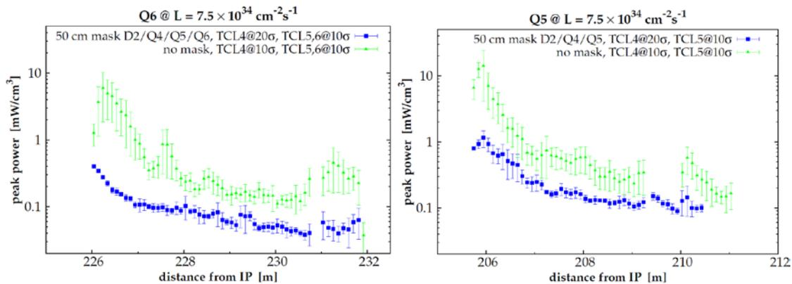
Figure 8: Peak power density induced by the collision debris in Q5 (left) and Q6 coils (right), assuming an instantaneous luminosity of  $7.5 \times 10^{34} \text{ cm}^{-2} \text{ s}^{-1}$ . The figure compares two alternative options: one with TCLs and masks and the second only with the TCLs (in all cases the TCL half gap is  $10\sigma$ ). Results apply to layout version HL-LHC v1.0 with round beams. Figure courtesy of L.S. Esposito et al. (from Ref. [17]).
