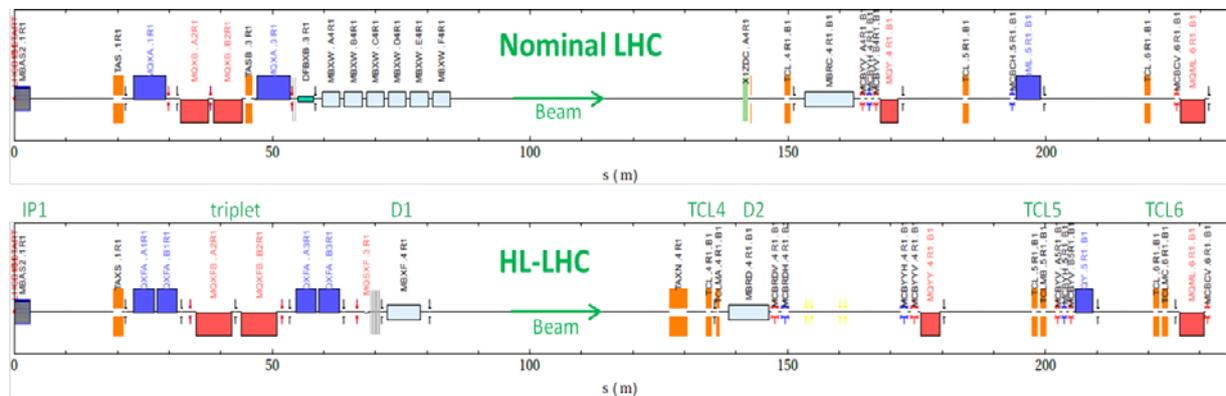
Figure 6: Layout of the elements seen by the outgoing beam in IR1 for the nominal LHC (top) and HL-LHC (bottom). The IR5 layout is equivalent. The longitudinal position of the interaction point is located at the zero of the x axis.
