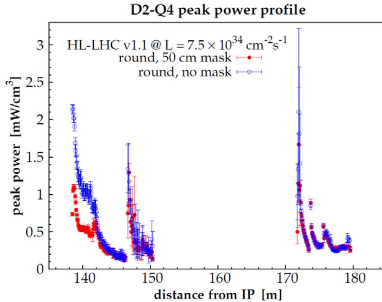
Figure 7: Peak power density induced by the collision debris in D2 and Q4 coils, assuming an instantaneous luminosity of  $7.5 \times 10^{34} \text{ cm}^{-2} \text{ s}^{-1}$ . The figure compares two alternative options: one with TCL-4 and TCLMA and the second only with TCL-4 (in both cases the TCL half gap is  $10\sigma$ ). Figure courtesy of L.S. Esposito et al. [35].
