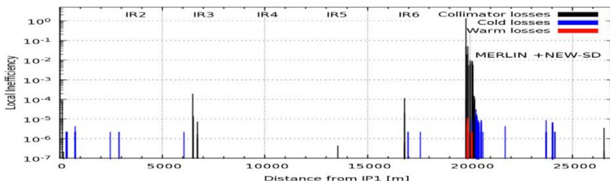
Figure 5: Losses around the ring, as simulated with MERLIN, for horizontal halo losses in the pre-squeeze optics configuration and using nominal collimator settings. The simulation includes a recently improved version of the scattering physics in the collimators. Figure from Ref. [14].
