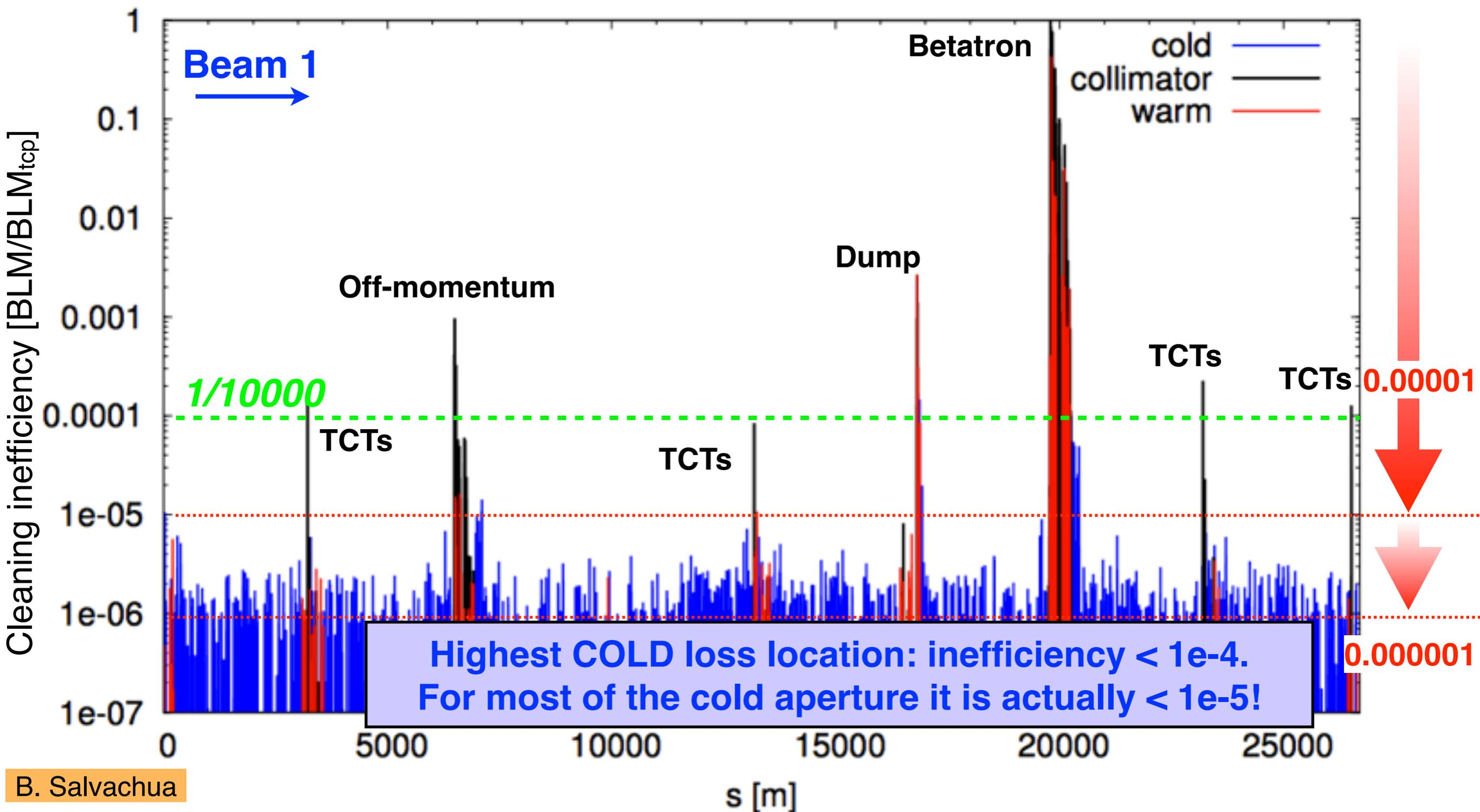
**2012-13: “tight” collimator settings (TCP gaps as at 7 TeV) for higher beta\*!
