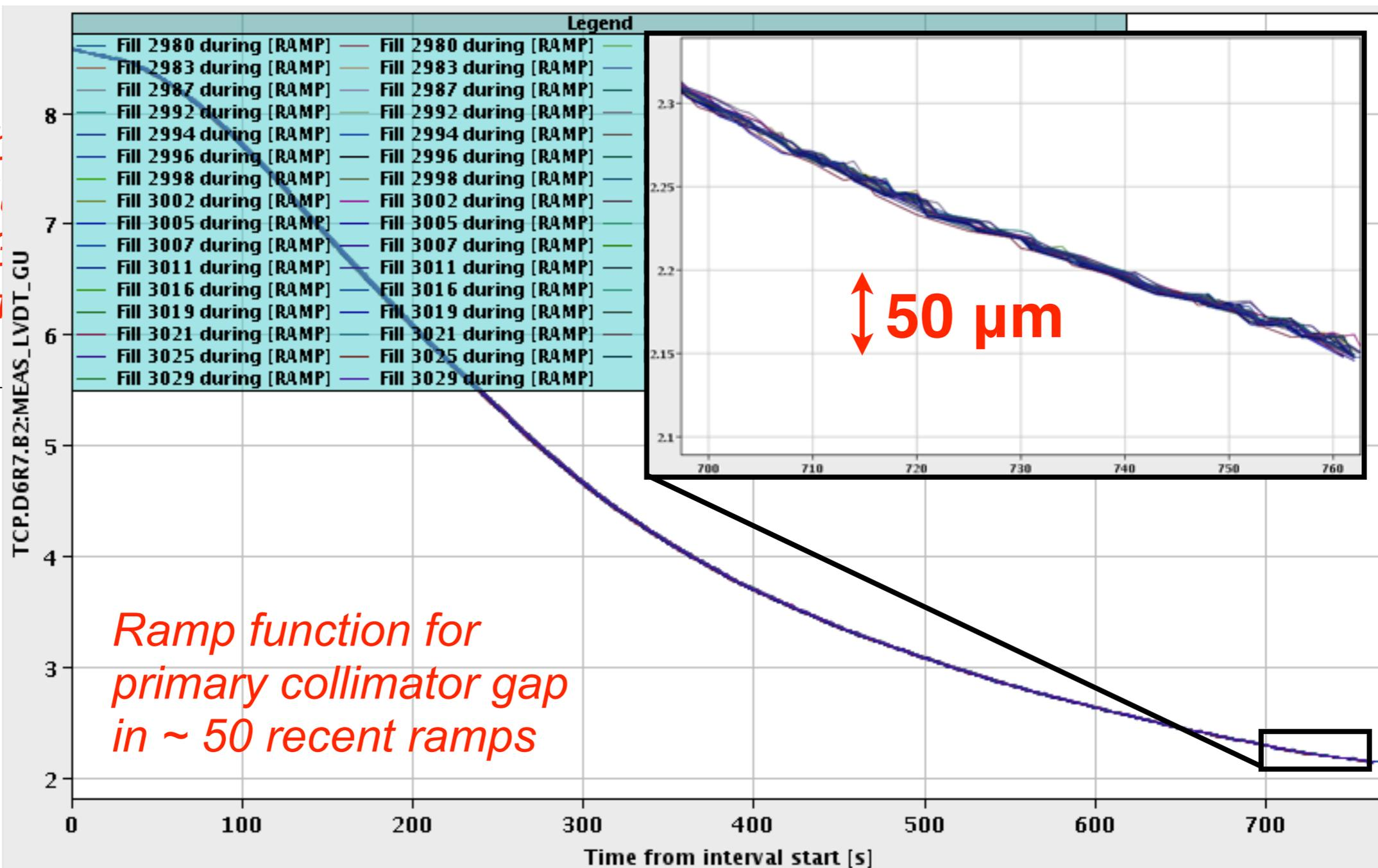
Ramp function for primary collimator gap in ~ 50 recent ramps
