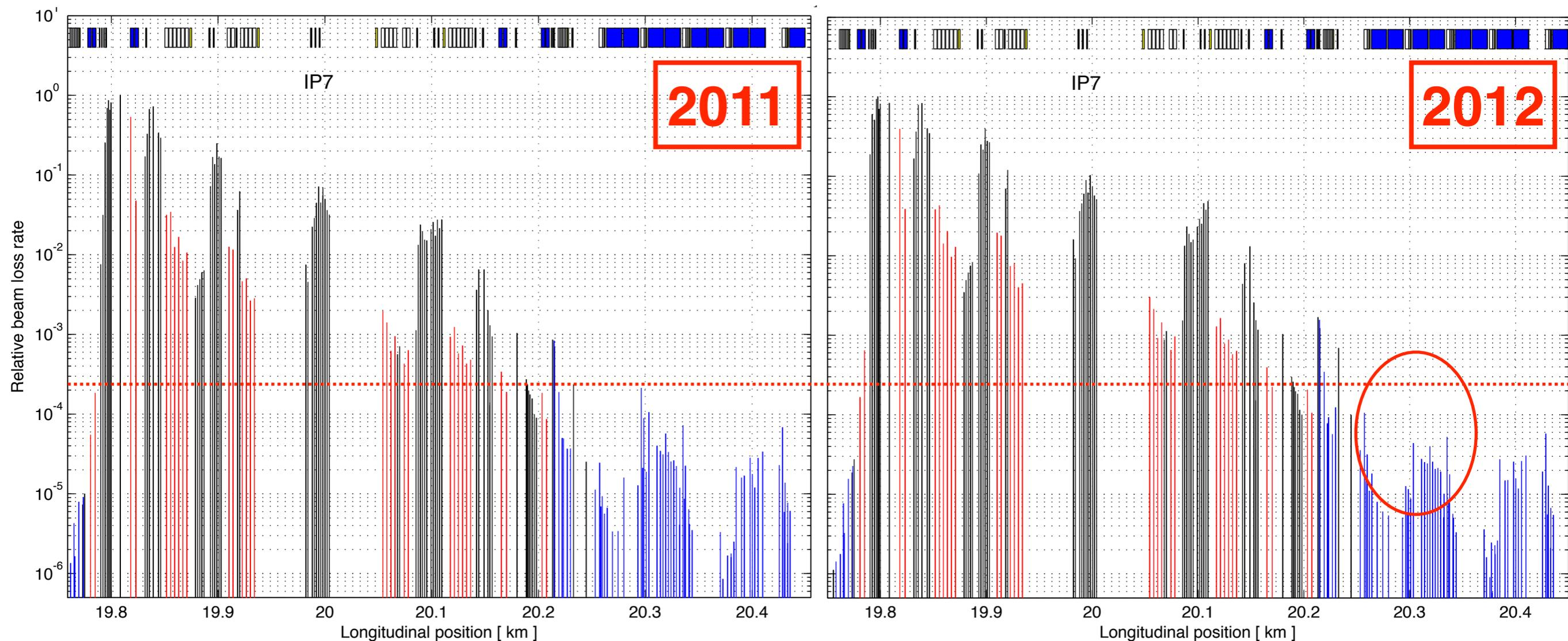
The local cleaning in the IR7 DS's was improved by a **factor ~5** compared to 2011, thanks to the deployment of collimator **“tight” settings**.
