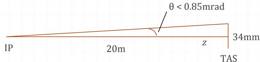
**Inelastic head-on collisions at the IP**
