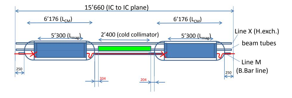
Collimator space reduced (w.r.t 2x5.3m 11T magnet+collimator option)
