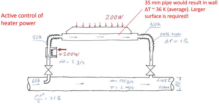
Dynamic pressure is sufficiently high; no need to add a restriction in line E
