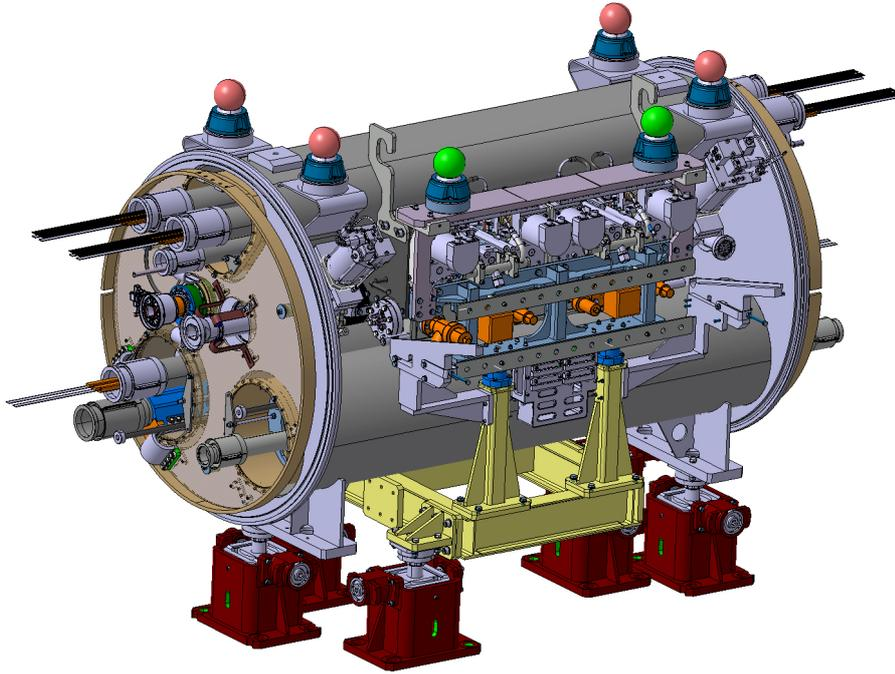
Figure 6 – The assembly to be installed between the two 11T dipoles, consisting of TCLD collimator, support, beam pipe for the other beam, and cryo-bypass. Courtesy of L. Gentini.
