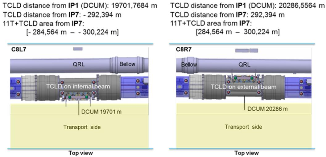
Figure 2 - Positions of new TCLD collimators in IR7. Figure taken from Ref. [12].
